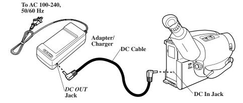
Since the battery must be charged before it can be used the first time, attach the adapter/charger to the camcorder.
